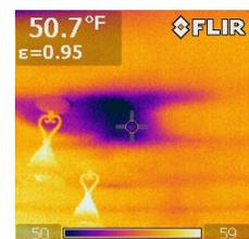
can show exactly how air is moving in a house. When partnered with a blower door, which places the house under pressure by typically pulling air out of a house (simulating an outdoor 20mph wind), it can aid in diagnosing where a house has the most critical energy losses and indicate what priorities should be made in creating a work order for the home.
