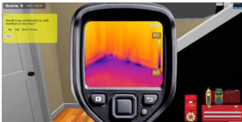
Users follow the simple instructions in the game’s tutorial to navigate throughout the house. They have a virtual toolbox including an IR imager, a moisture meter, and a sensor <sup>1</sup>. Scanning the home with either the IR or the moisture meter reveals hot spots, indicated by dots on the walls, floors or ceilings. Users select the IR from the toolbox and point it at the spot to reveal the multiple-choice question.
